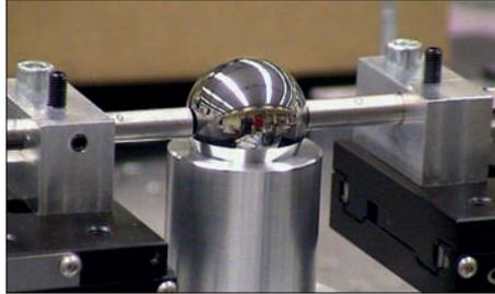
techniques to measure hysteresis curves in the normal displacement (perpendicular to the surface) of a sliding object as it is pushed along. They tested various materials (paper, plastic and brass) at different speeds,
