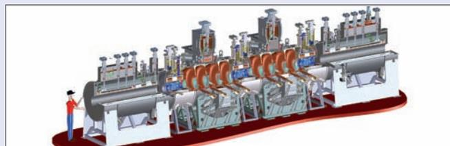
Fig. 4. Cutaway rendering of the international Muon Ionization Cooling Experiment. The muon beam enters from the bottom left of the figure. (Image credit: A DeMello/LBNL.)
