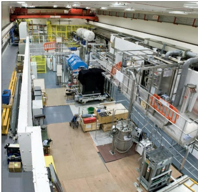
Fig. 5. The MICE Hall in June 2011. The ISIS synchrotron lies behind the wall at the back. The downstream quadrupoles (blue) are visible in front of the concrete shielding (white), with a TOF hodoscope for particle identification immediately after the final quadrupole. This hodoscope is followed by the lead-scintillator section and the prototype electron-muon ranger. In the foreground are the prototype liquid-hydrogen delivery system and R&D cryostat. (Image credit: S Kill/STFC.)
