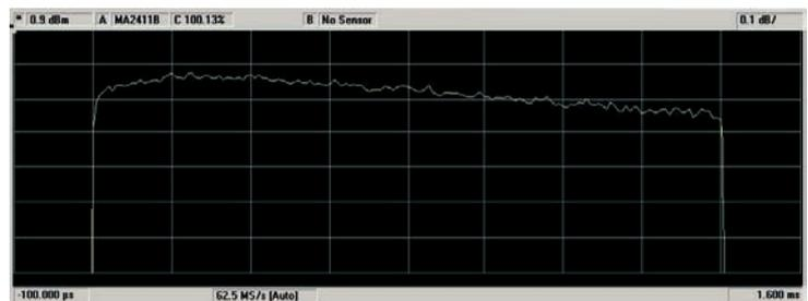
Typical 1.6ms 1kW pulse @ 1.3GHz
